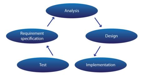
Illustration 3.1: The iterative design makes sure that product development adheres to results of user tests of previous prototypes.
