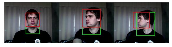
Illustration 4.3: Face detection using OpenCV's Haar cascades. The images show tracking with a combination of frontal and profile cascades. The red rectangles are the original bounding boxes produced by OpenCV and the green ones are scaled versions of these bounding boxes, made to fit the entire skin region.
