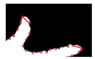
Illustration 4.2: By calculating the angles between the points along the contour, it is possible to find the narrowest angles and identify these as fingertips. In the picture above, the two narrowest angles are highlighted with lines to illustrate the angle. The image is an actual result from the application implemented.
