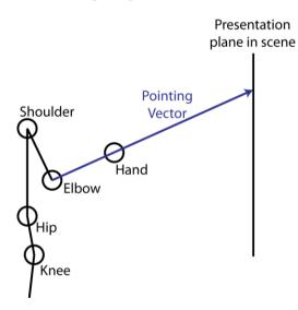
Illustration 8.1: Pointing in the skeleton tracking approach happens through creating a vector from elbow, through the hand and onto the presentation plane in the Unity scene.
