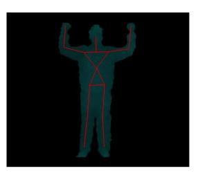
Illustration 7.1: In order for the NITE library to correctly initialize the skeleton, the user is required to stand in the pose shown here. After a few seconds the NITE library will have mapped the skeleton to the user.
