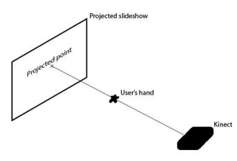
Illustration 5.1: Pointing is achieved by tracing a line from the Kinect camera to the slideshow projection, which passes through the presenter's hand.
