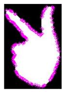
Illustration 6.3: Having found all the points along an OpenCV contour produces quite an extensive list of points. All the magenta colored circles are points along the contour, returned by OpenCV.
