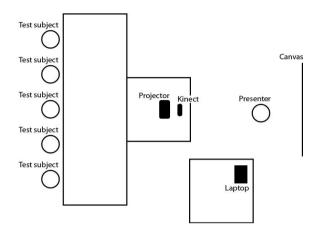
Illustration 9.1: The setup for the test of the presentation tools. The presenter would be standing in the position depicted above only for the gesture based test case. For the traditional presentation he would be standing at the laptop to be able to control the presentation.
