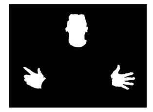
Illustration 4.1: The blobs seen in an incoming image after skin segmentation has been completed. The face and hands are the only visible parts left. This is an ideal situation and the image is not a result of the final application.
